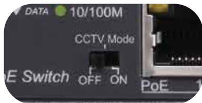
CCTV Mode Switch
